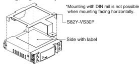
Note: 1. Improper mounting will interfere with heat dissipation and may occasionally result in deterioration or damage of internal parts. Use the product within the derating curve for the mounting direction that is used. Do not use the Power Supply mounted in any way not shown above.
