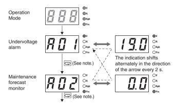
Note: 1. When undervoltage alarm is indicated: Press ⊋ → output load indication When the maintenance forecast monitor or overheat alarm is indicated: Press ⊋ → undervoltage alarm indication
