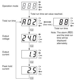
The accumulated value of the operating time of the Power Supply is displayed as the total run time.  $\Box$  (kh) will be displayed initially after purchase and then the display will advance in 1-kh steps as the operating time accumulates. When the total run time reaches the preset alarm set value, the alarm ( $\Box$  and the total run time will be displayed alternately and a transistor ((12) total run time output terminal (kh)) will output the status externally.
