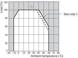
**Note: 1.** Using side mounting bracket for right-side mounting (excluding 240-W Models).
